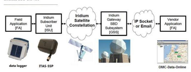
SBD messages are transmitted to an Iridium server (GSS: Gateway Short Burst Data Subsystem) and you can ask your Iridium provider to pass SBD messages to an e-mail address of your choosing or via directIP to an IP-address/domain and TCP-port of your choosing. When using your own software you have to either pick-up and import the e-mails or implement a TCP-server to receive SBD messages.
