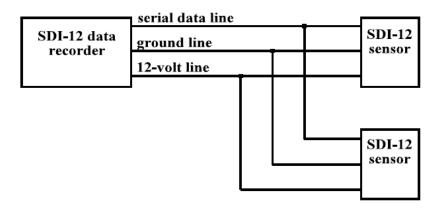
The wiring length between a sensor and the data-recorder must not exceed 60 meters. The maximum number of sensor connected to a SDI-12 bus is limited to 10. The data logger is protected against transients on the SDI-12 bus.
