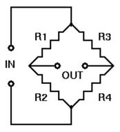
Given, all R's are the same the output voltage will be 0 Volts. In practice, one of the resistors is replaced by a variable resistor (often a strain gauge). By varying the resistance of this resistor, the bridge will be "unbalanced" and there will be an output Voltage, other than 0 Volts. To enable the circuit, the bridge has to be powered by a very stable reverence Voltage, often called "Excitation Voltage". The OMC-042 has an Excitation output for this purpose.
