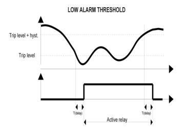
So, the entry of an alarm state is NOT affected by a hysteresis. Hysteresis is only used for switching back to the normal mode. The amount of hysteresis has an effect on the "sensibility" of the alarming. It is strongly advised to use a certain amount of hysteresis to prevent from multiple alarming warnings. The amount of hysteresis is determined by experience and information from the sensor.
